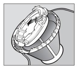
To clean the underside of the filter, the flap must be opened:
